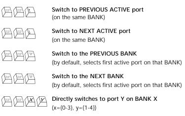
You can switch directly to any port by giving the OmniView™ SE the BANK and PORT numbers. For instance, if you press [SCROLL LOCK] [SCROLL LOCK] [2] [2], the computer on PORT 2 of the OmniView™ SE set to BANK 2 will be selected. In the diagram below, that is PC # 8. Hence, if you only have one OmniView™ SE, the first key (X) must be "0".
